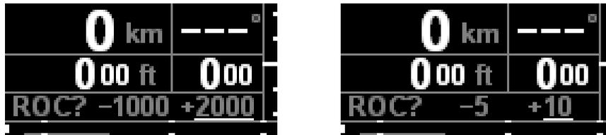
Depending on the selected unit the rate of climb maximum scale value (second marking) can be chosen to be  $\pm 1000$  ft/min resp.  $\pm 5$  m/s or to be  $\pm 2000$  ft/min resp.  $\pm 10$  m/s.
