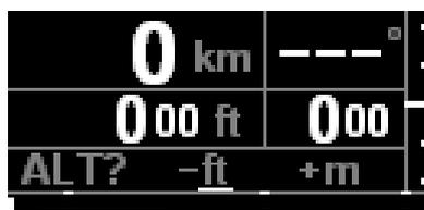
The altitude can be provided in feet (ft) or in meter (m). An additional cue for the values given in feet (ft) are the downsized last two digits.
