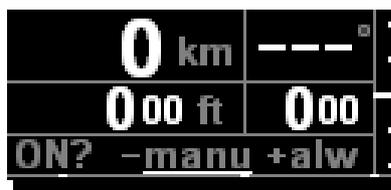
This configuration option defines whether the device shall be switched on manually (**manu**) or whether shall turn on automatically whenever power is supplied (**alw**).
