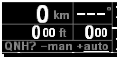
This option allows to define whether the device initiates one automatic QNH determination each time after being turned on, or not.
