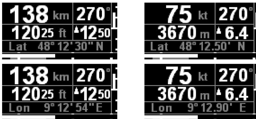
The format in which the coordinates are given be configured to be either *Degree°Minute'Second* or *Degree°Minute.Centiminate*' (see 2.5.2.8).
