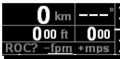
The rate of climb is provided either in meter per second (**mps**) or in feet per minute (**fpm**). The selected unit is reflected by the respective format of the numerical value:
