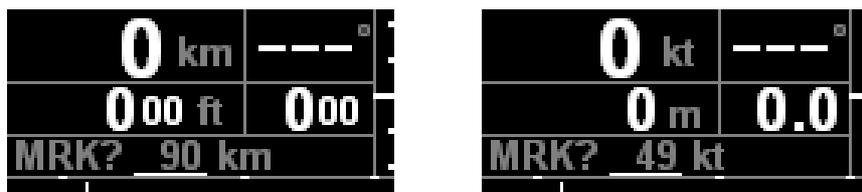
It's position is adjusted with the setting buttons **- QNH +**. The unit of this speed value is the same as the one configured for the indicated airspeed (IAS) **km/h** or **kt**.
