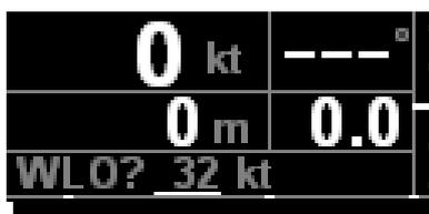
The value of the lower limit is adjusted with the setting buttons **- QNH +**. The unit of this speed value is the same as the one configured for the indicated airspeed (IAS) **km/h** or **kt**.
