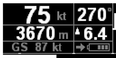
After pressing **INFO** again the groundspeed is shown in the third line. The groundspeed is always shown in the same unit as the airspeed (IAS) is indicated. This unit is configurable to be **km/h** or **kt** (see 2.5.2.7).
