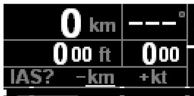
The airspeed is either provided in **km/h** or in **kt**.
