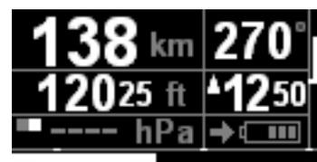
While the automatic QNH-determination is in progress (this requires a valid GPS position), the numerical value for the QNH is substituted by „----“. During this indication the last QNH value is
