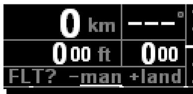
It is possible to select having the flight time displayed only after being selected manually (“man”) or additionally automatically after each landing (“land”).
