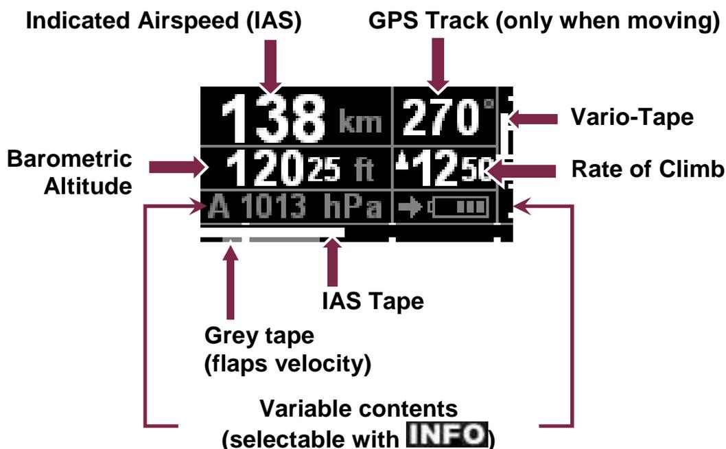
While essential informations like airspeed, altitude, track and rate of climb are displayed permanently, the content of the third line is selected out of a predefined set (described in section 2.3.2).
