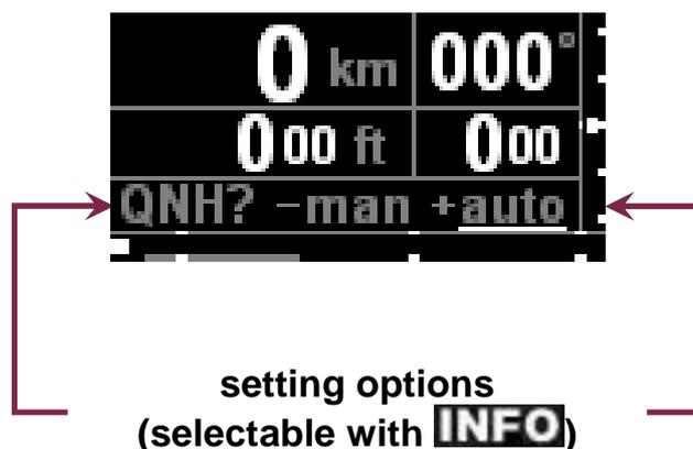
From normal operation mode the settings mode can be accessed by pressing **SET** long.
