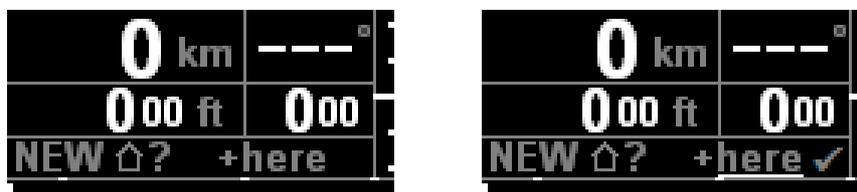
When having GPS reception, the current position can be stored as new home airfield location for the return-home aid. The successful operation is indicated by displaying a check mark.
